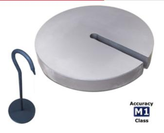
Disc weights suitable for legal metrology applications and the industrial sector and fully customisable. They have a groove and relief to allow them to interlock and keep them concentric; the slot allows them to be positioned on the bar. Their tolerances are those provided for OIML M1 class masses and therefore allow these weights to be used for the control and calibration of scales and class III instruments up to 10.000e.
